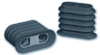
Designed for gripping 750 ml bottles, the VSBO and VSBO+ suction cups are available with a new sensing valve (V3 version) ensuring an airtight vacuum network if a bottle is missing. This new technology gives a greater sensitivity in opening the valve and placing the suction cup under vacuum once contact is made with bottle.
