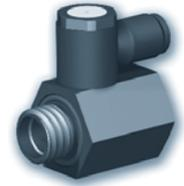
The CSP series safety valve is a useful safety device. In the event of loss of vacuum or emergency stop it maintains the vacuum in the suction cup. Release is obtained by connecting the ancillary coupling to the pressure supply.
