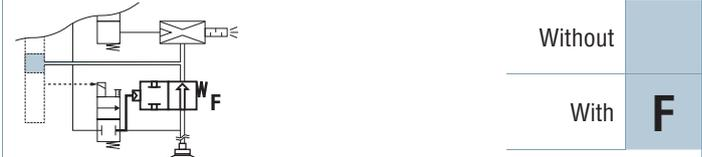
The powerful blow-off option allows you to release the product quickly. Isolation valve **F** directs the entire blow-off flow to the vacuum pad. The option is only available with LEM+ modules equipped with a blow-off regulation: Version LEM\_\_X\_\_SV... and LEM\_\_X\_\_VV...
