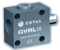
Due to its ultra light and compact nature, the GVRL ejector can be easily integrated onto automated, high-speed grippers. Its tough aluminum design is reliable and allows the GVRL to be mounted directly to the suction cup.
