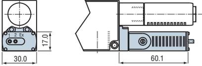
For use in fully pneumatic applications or explosive environments. The vacuum switch enables a pressure data message to be given when a vacuum threshold is reached.
