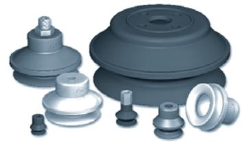
The VSAG series 1.5 bellows suction cups are recommended for gripping concave or convex products as well as sensitive products due to the cushioning effect of the bellows. The bellows also compensate for height variations in product gripping.
