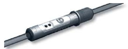
Due to their lightweight and compact design (only 7 to 13 g depending on the version), the "just plug it in" CIL ejectors can be easily integrated into the compressed air network and very close to the suction cups, even in the most inaccessible parts of the machine.
