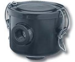
The FVI range is compatible with pneumatic vacuum generators (venturi) or electric vacuum pumps (the FVI 2 model is suitable for a suction turbine). Each filter is fitted with an interchangeable cartridge treated to guarantee long life expectancy for the whole unit. The filtering element consists of a 5 micron filter (made of paper for version C), which is sufficient to protect pumps and venturi under normal operating conditions.
