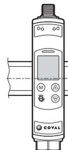
For a static mounting (for example, in a cabinet), a module can be clipped onto a DIN rail. For this purpose, the module must first be equipped with an individual plate for fixing onto a DIN rail, to be ordered separately:
