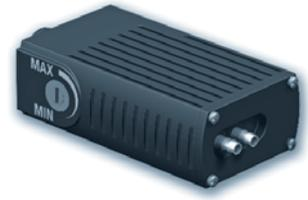
The PSE 100 P series vacuum switch with pneumatic output allows the vacuum level in the system to be checked by means of a patented system. This vacuum switch exists in two versions: NO version recommended for the "air saving" function on a venturi and NC version for the "safety" function (object detected, etc.) and "SFC signal".
